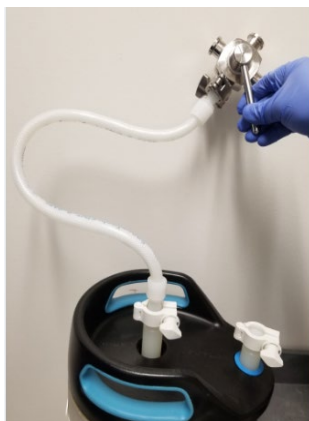
Figure 2. Stainless Steel valve connected to tubing
