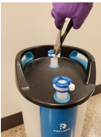
Figure 1. SaniSure Clamp Removal
